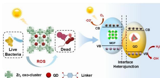
Fig 1 : Scheme of the photocatalytic effect of MOF/QDs composite for effective bacteria-killing under NIR-light irradiation
